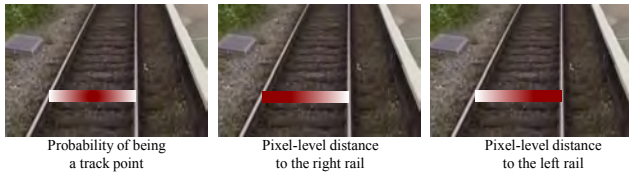
Fig. 3. Expected regression outcomes of the first design of the regression branch in a sample rail area of the input image. Each outcome is a 1-channel heatmap. Here, the heatmap value gets larger as the color goes darker.
